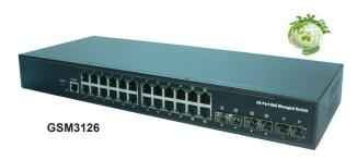
**Waters Network Systems' GSM3126** switches deliver reliable intelligent 10/100/1000Base-TX connectivity services from the core to the edge. The GSM3126 models provides the application intelligence, manageability and performance to support IP data, voice and video deployment for today's most demanding LAN applications. Four combo slots are available for either 100Base-FX or 1000BaseSX/LX modules.
